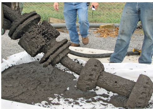
Figure 2: Pig over-loaded with black powder.
