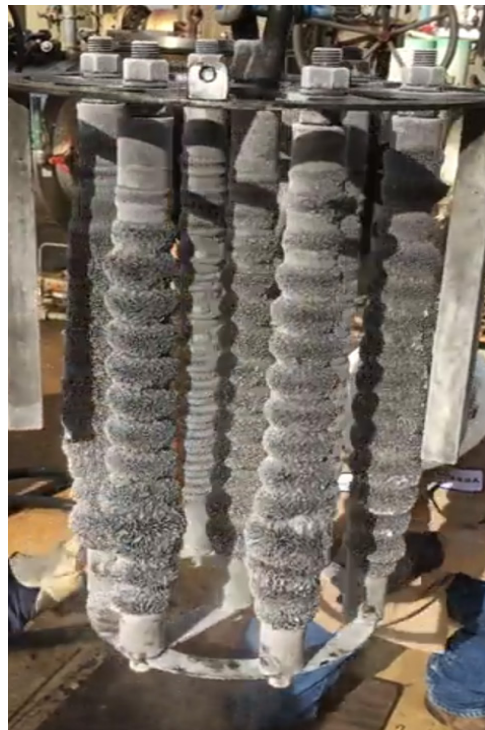
Figure 5: Black Powder captured on magnetic elements.
