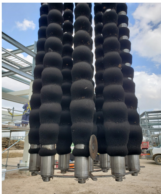
Figure 4: Black powder captured on magnetic separator elements.
