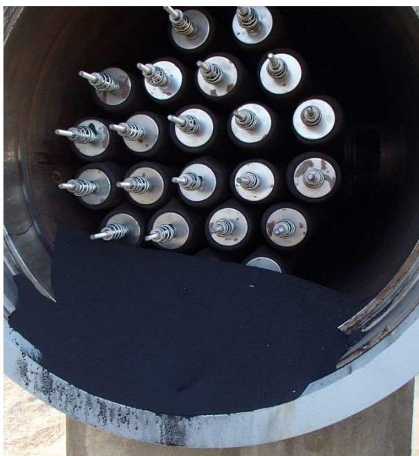
Figure 3: Uncaptured black powder built up in a conventional filter housing.
