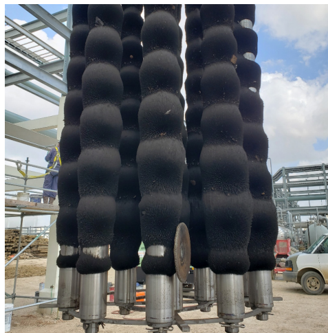
Figure 2. Black powder captured on a magnetic separator system.
