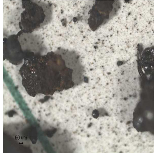
Figure 3. Black powder particulate under microscope.
