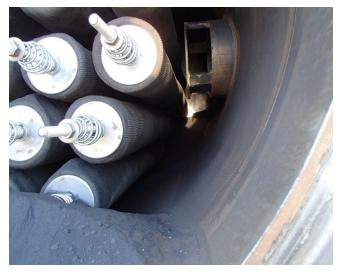
Figure 2. Contamination not captured by conventional filters.
