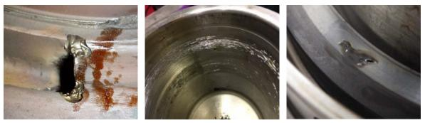
Figure 1. (a) Centrifugal pump wear. (b) Magnetic drive pump wear. (c) Mating ring wear & residue.
