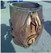
Figure 3. Examples of damaged strainers.
