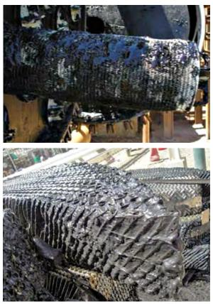
this passivation layer may be removed mechanically by abrasion or erosion, a chemical reaction with hydrogen cyanide (in refineries), or by dissolving in the amine solution itself. Abrasion or erosion can occur when hard particles circulate within the amine, abrading or knocking the iron sulfide loose from the underlying steel<sup>1</sup>.
