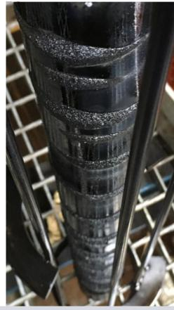
BPS magnetic separator installed in the HDS amine system during testing, as well as contamination captured after 2 weeks of testing.
