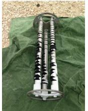
of Black Powder (BP) in their 6" propane line. The BP was damaging their valves, meters and pump components, and degrading the liquid propane quality.
