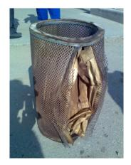
the entrained liquids from the gas, increasing the amount of liquid trapped in the depth media element, and causing entrained liquids to continue down the line.
