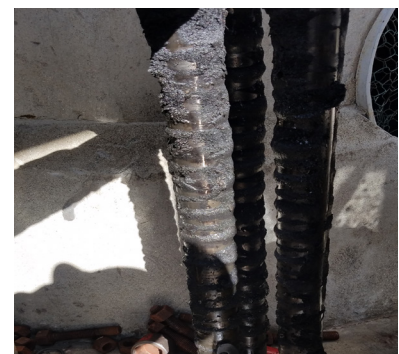
Contamination collected from finished distillate product: diesel fuel and kerosene, after 6 weeks of operation. The magnetic separator systems cleaned the product to the standard that it did not require clay-filter color removal.
