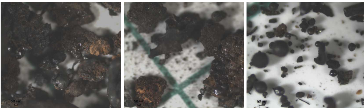
Figure 10: Microscopic images of a black powder sample pulled from a natural gas dispenser feedline via SEM.
