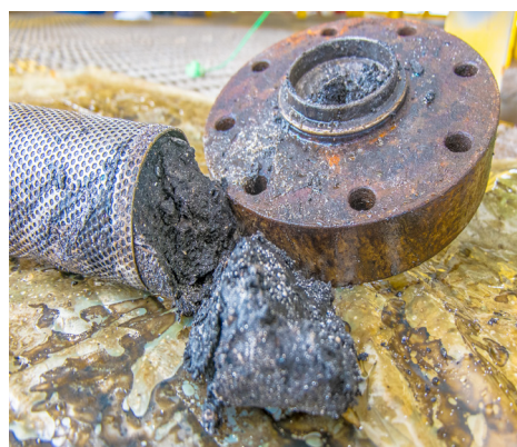
Figure 12: Conventional filter plugged off with black powder.
