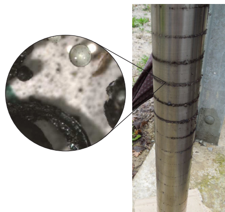
Analysis of the contamination collected indicated high levels of non-ferrous particulate caught by the magnetic elements
