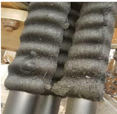
Black powder removed from the suction of a kerosene product pump.
