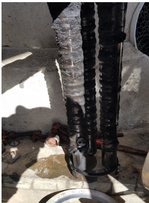
Black powder collected after six weeks of operation.
