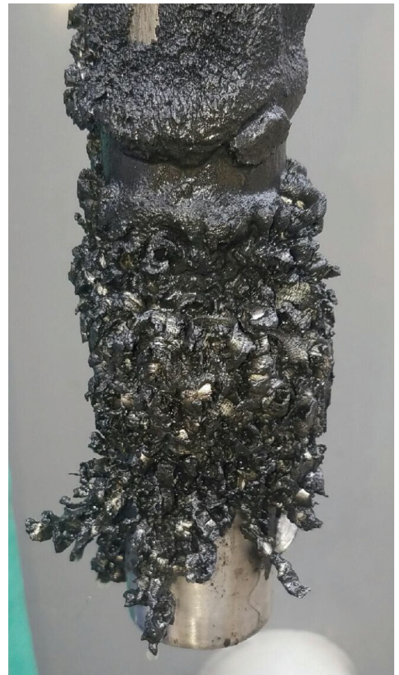
Figure 1. Black Powder collected on the first Magnetic Separator element after 18 hours of operation.
